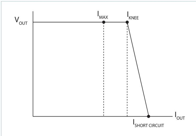
Figure 3.1 — Typical Maxi, Mini, Micro current limiting
