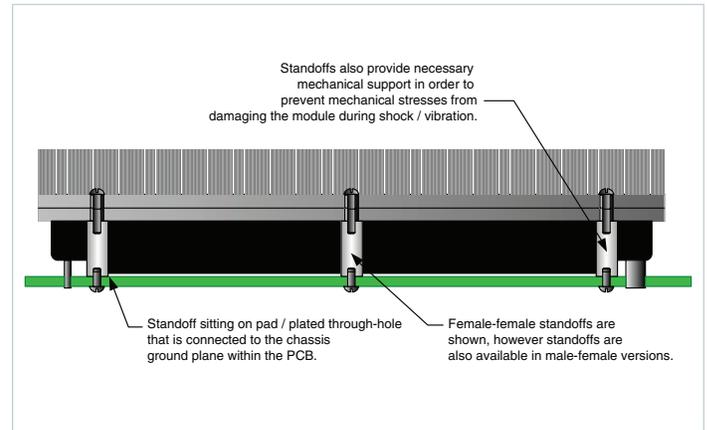
Figure 3.3 — Recommended mounting method using standoffs
